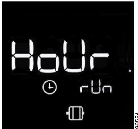
Figure 29: Running hours screen
