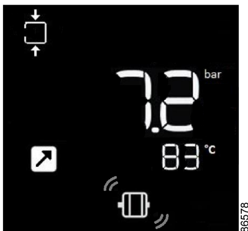
Figure 25: Main screen with shutdown indication, motor overload
