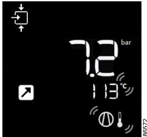
Figure 20: Main screen with temperature outlet warning
