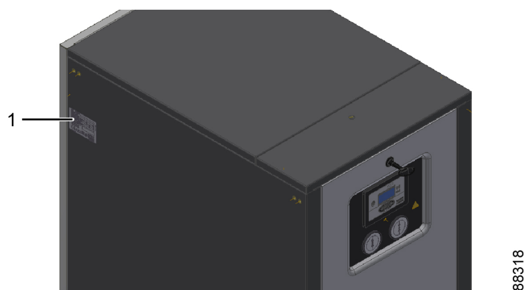
Figure 4: Location of the identification plate on the dryer
