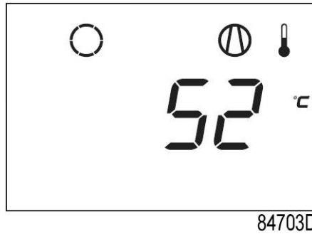
Main screen with temperature (stopped compressor)
