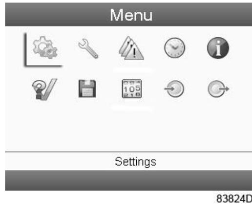
Using the Scroll keys, move the cursor to the Settings icon and press the Enter key. Following screen appears:
