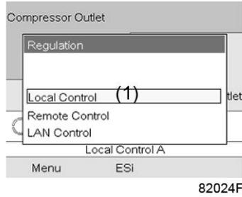
After selecting the required regulation mode, press the Enter button on the controller to confirm your selection. The new setting is now visible on the Main screen. See section [Icons used](#) for the meaning of the icons.
