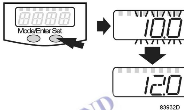
Numerical values are incremented continuously. If the value is to be reduced: let the display move to the maximum setting value. Then the cycle starts again at the minimum setting value.
