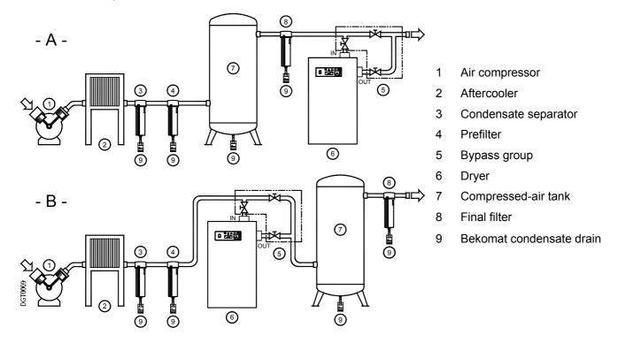
Installation **type A** is recommended when the total consumption corresponds to the throughput rate of the compressor. Installation **type B** is recommended when the air consumption constantly varies, with peak values which considerably exceed the throughput rate of the compressor. The storage capacity of the tank must be dimensioned in such a way that a possible short-term high air demand (peak air consumption) can be compensated.
