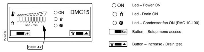
The DMC15 displays DewPoint temperature, controls the condenser fan activation and the timed drainer.
