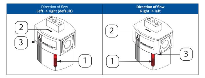
The housing head and the housing body are equipped with a double-start trapezoidal thread. The direction of flow of the filter can be adapted to the direction in the pipe by turning the housing head through 180°. The direction of flow is indicated by arrows [2] and a raised marking [3] on the housing head. These must be aligned as shown. The safety slide [1] must always be in an easily accessible position on the front.
